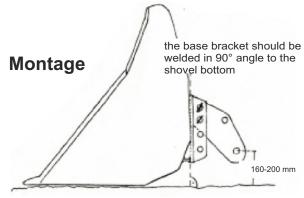
The basic bracket shall be welded on the back side of the shovel do to this, the shovel should be set down on the ground in working position! (see sketch) Now plug in the mounting arm in the top hole of the basic bracket.
