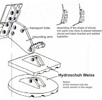
the mounting arm can be fitted in different hole high, if the ground level has different height!
